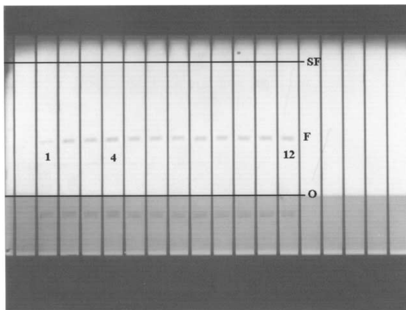
Figure 1. Chromatograms obtained in the duplicate analysis of four 10 mg famotidine tablets (Table 1, Brand 1, Tablets 1–4) on a channeled silica gel plate with concentrating zone by the described HPTLC-densitometry method. The plate was photographed under 254 nm UV light with a Camag VideoStore Image Documentation System. Key: SF, mobile phase front; O, origin; lanes 1–4: famotidine (F) standards; lanes 5–12: duplicate aliquots of the four sample extract solutions.
